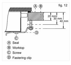
Note: It is essential that the sealing washer is placed beneath the hob's rim. If it is not placed there, the worktop could suffer extremely high temperatures.
