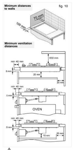
When installing units or appliances above the hob, the hob should be protected by a board so that the glass cannot be damaged by accidental blows or heavy weights.
