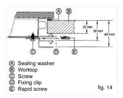
Hob model CGC 4G AI AL is mounted by inserting the quick nuts into the holes where the screws go (see fig. 14) and then attaching the appropriate clip, depending on the worktop's thickness (20, 30 and 40 mm) and tightening the screws until it is firmly fastened.
