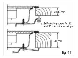
On models CG.1 4G and CG.1 3G 1P, the clips should be fixed as shown in figure 13, depending on the thickness of the worktop.
